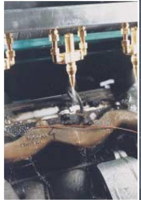
Sprayvectors introduce 2-20 PSIG (0.14-1.4 Bar) filtered liquids through a 1/4" NPT port. They can spray liquids with viscosities up to 1100 CPS for fogging and atomizing applications. Liquids with viscosities up to 100 CSP are suitable for humidifying. Large internal passages eliminate
