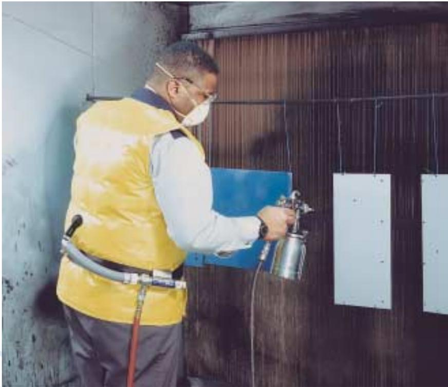
Unlike “ice pack” type vests, the PAC offers consistent, continuous and controllable cooling to minimize heat stress and increase worker productivity in hot surroundings. The durable, plasticized PVC vest allows full range of motion with no airflow restrictions and can be worn under welding leathers or protective clothing. Both large and extra-large vests are available, each featuring a collar that can be unfolded to deliver tempered air flow to the neck and face.
