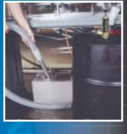
Automatic safety shutoff valve prevents overflows
