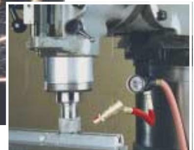
Nozzles are an excellent replacement for open copper tubes, flex-line and other nozzles not designed to save air. A full range of styles is available, with designs compatible to most installations.
